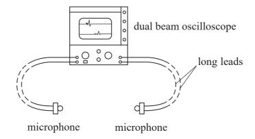
The student will make a noise near one of the microphones. The oscilloscope can display the signals from both microphones as traces on the same screen. The student will observe the difference between the two stationary traces.
